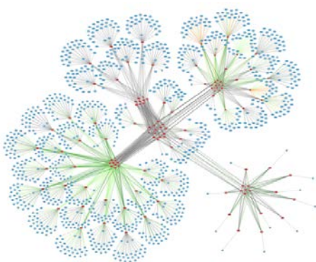
Network View of Ohio Supercomputer Center (OSC) with 3 heterogeneous clusters all connected to the same InfiniBand Fabric
