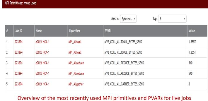
User can see which algorithms are used for MPI operation and interplay of MPI modules
