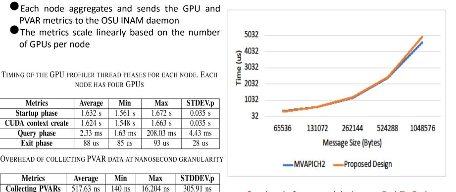
Overhead of proposed designs on End-To-End Performance MPI Allreduce for different message sizes
