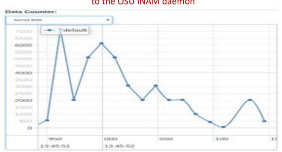
Screenshot of NVLink Metrics chart for TensorFlow. The X-axis represents time and Y-axis represents the link bandwidth utilization
