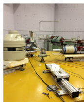
Fig. 6 The array of HPGe detectors.
