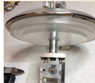
Fig. 3 The ^{112}\text{Cd} target used in this experiment.
