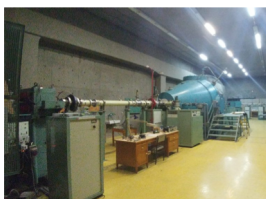
Fig. 5 The 5.5 MV Tandem accelerator at NCSR "Demokritos".
