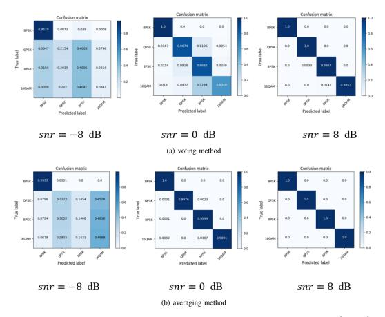
Fig. 6. Confusion matrices of CNN using (a) relative majority voting method and (b) arithmetic mean method when  $snr \in \{-8,0,8\}$  dB.
