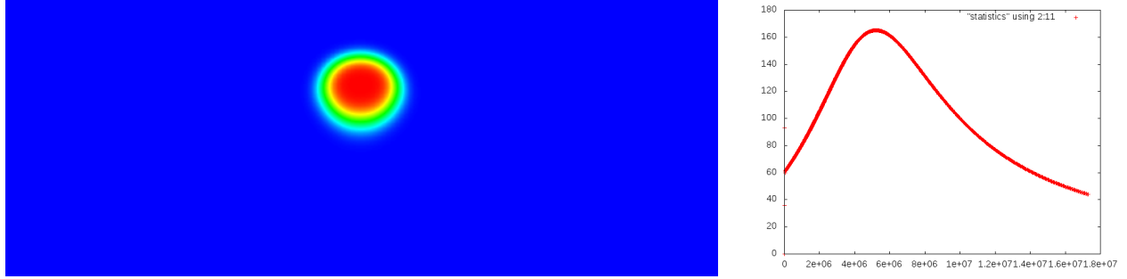
Figure 25: Evolution of surface topography due to a rising blob. On the left is a snapshot of the model setup. The right shows the value of the highest topography in the domain over 18 Myr of model time. The topography peaks at 165 meters after 5.2 Myr. This cookbook may be run with the cookbooks/free-surface.prm input file.
