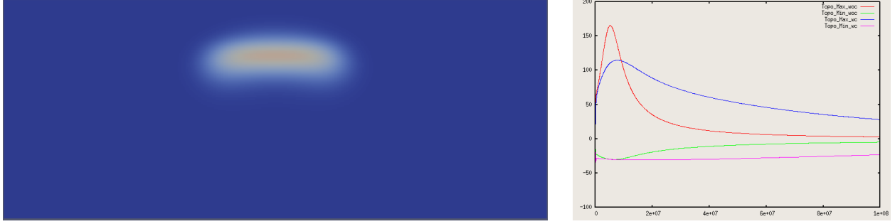
Figure 26: Adding a viscous crust to a model with surface topography. The thermal anomaly spreads horizontally as it collides with the highly viscous crust (left). The addition of a crustal layer both dampens and delays the appearance of the topographic maximum and minimum (right).
