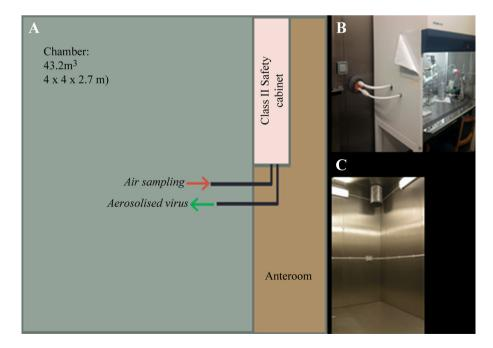
**Figure 1.** Experimental chamber and anteroom (A) containing the BSC II cabinet. (B) Collison nebulizer source 'aerosolized virus' outlet (green arrow) and the 'air-sampling' inlet to the SKC BioSampler (red arrow). (C) Interior of the stainless steel experimental chamber. (For interpretation of the references to colour in this figure legend, the reader is referred to the online version of this article.)
