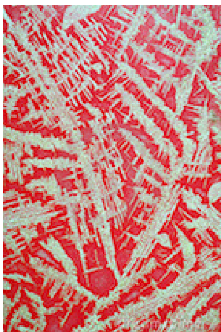
Photo 3. Dried material after ethyl acetate extraction of Caloplaca inclinans thalli. The material formed flat red crystals on the surface of the dish.
