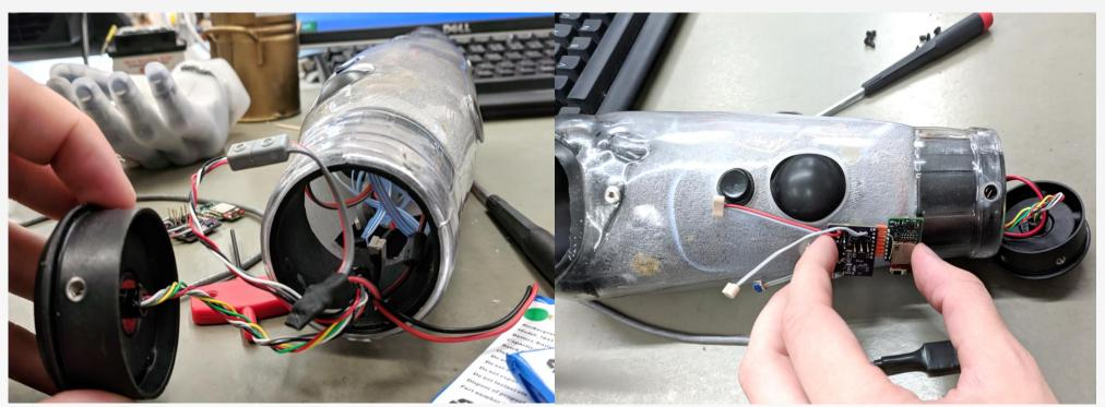
Figure 3 – Opening of the socket
