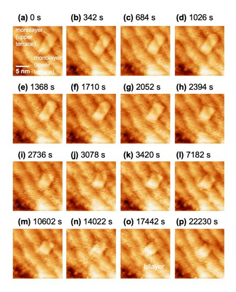
**Figure S3** Sequential STM images showing the NaCl bilayer formation on the NaCl monolayer island on Au(111) at room temperature. (a) An STM image focused on the NaCl island indicated by F in Figure 4. (b)-(p) The STM images obtained at the same area of (a) after the indicated time. The NaCl monolayer on the upper terrace was transferred to the NaCl island on the lower terrace forming the bilayer. All STM images were obtained by  $V_s=0.5$  V and  $I_t=0.5$  nA.
