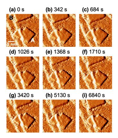
**Figure S1** Sequential STM images showing the stability of the NaCl bilayers on Au(111) at room temperature. These images are the same as those in Figure 5, but displayed via the derivative processing. (a) An STM image focused on the NaCl bilayers indicated by A and B in Figure 4. (b)–(i) STM images obtained at the same area of (a) after the indicated time. All the STM images were obtained with  $V_s=0.5$  V and  $I_t=0.5$  nA.
