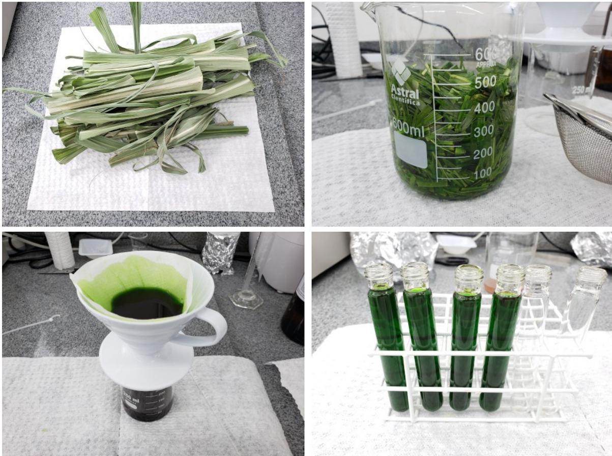
**Figure 6.10:** Sugarcane dye extraction. Leaves (upper left), after blending (upper right), filtration (lower left) and dye before centrifugation (lower right).
