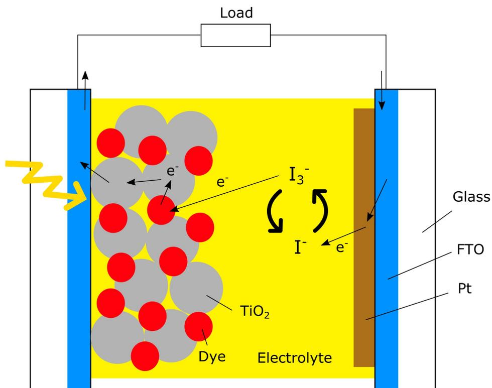
**Figure 2.1:** Construction diagram and working principle of a DSSC.
