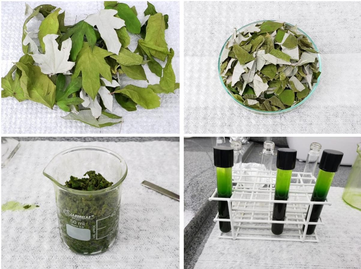
**Figure 6.6:** Dye extraction from embaúba-vermelha. Leaves (upper left), cut leaves (upper right), ethanol blend (lower left) and dye before centrifugation (lower right).
