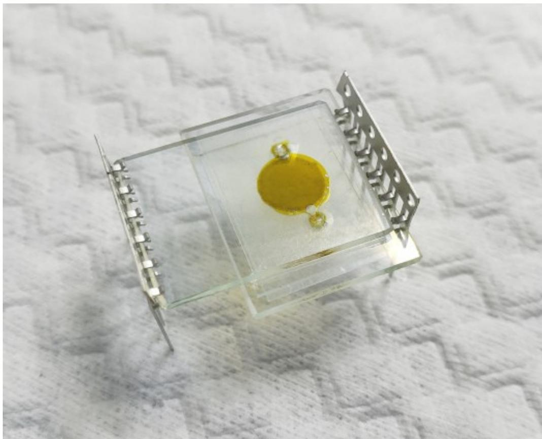
**Figure 5.3:** Scheme and picture of NDSSC fabricated.
