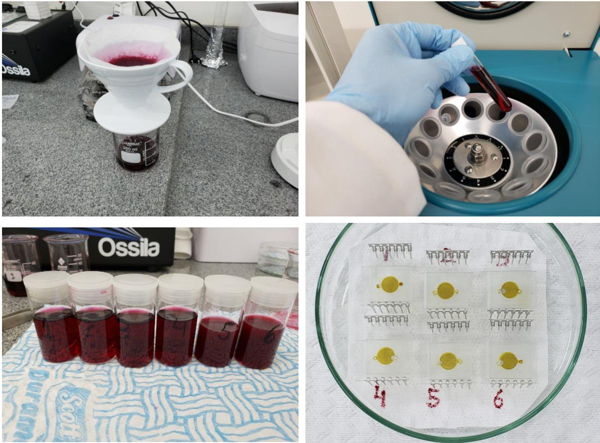
**Figure 6.2:** Blackberries dye. Extract filtration (upper left), centrifugation (upper right), cells sensitizing (lower left) and fabricated cells (lower right).
