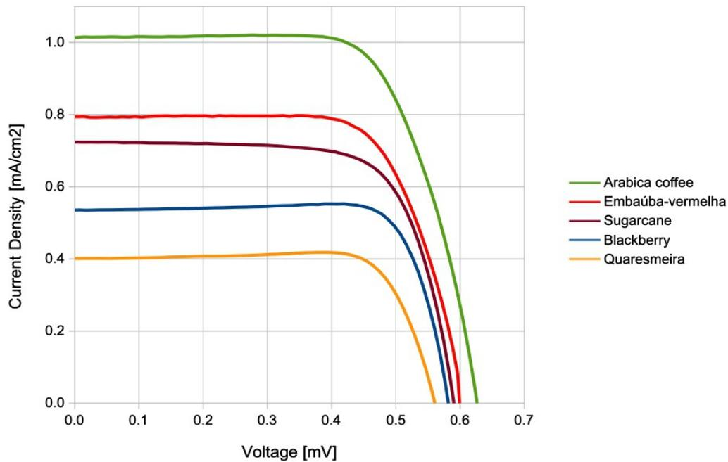
**Figure 6.11:** JxV curves of the best cells of each plant.
