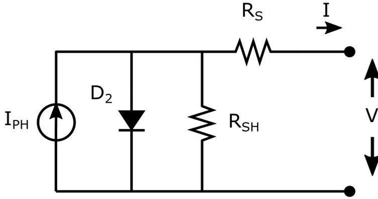
**Figure 2.4:** One diode model of a photovoltaic cell, including DSSCs.
