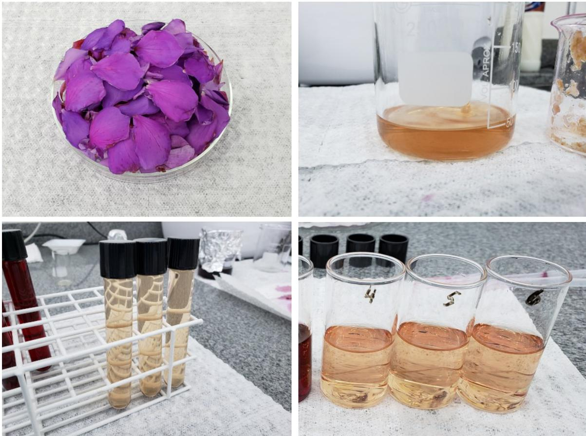
**Figure 6.4:** Dye extraction and cells fabrication from quaresmeira flowers. Petals (upper left), filtered extract (upper right), tubes after centrifugation (lower left) and sensitization (lower right)
