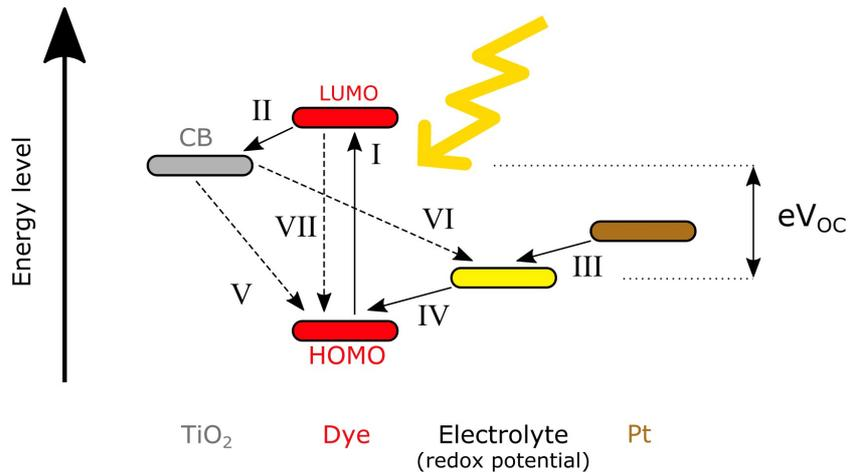
**Figure 2.2:** Energy levels diagram of an ideal DSSC [7][5].
