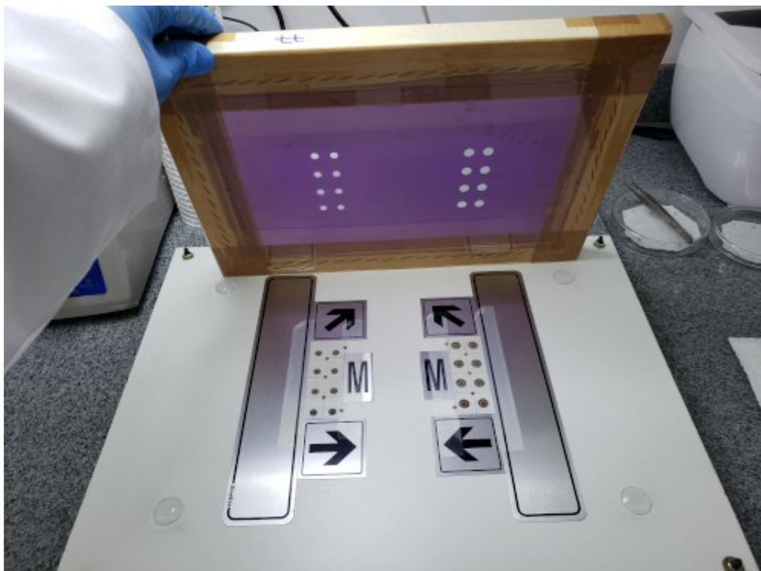
**Figure 5.5:** Pictures of the screen printing template and screens.
