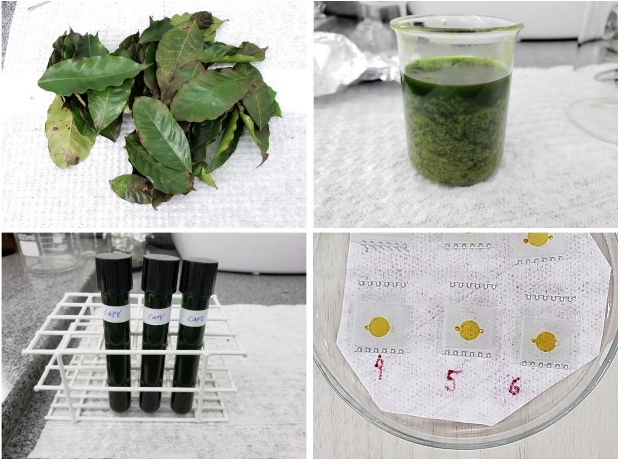
**Figure 6.8:** Dye extraction from arabica coffee. Leaves (upper left), extract after blending (upper right), dye centrifuged (lower left) and cells fabricated (lower right).
