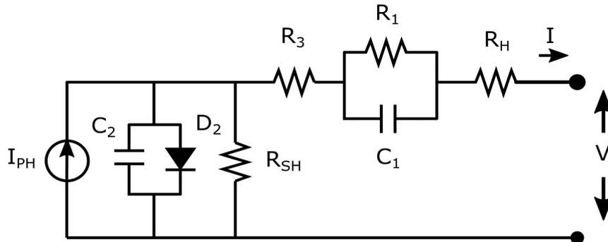
**Figure 2.3:** DSSC equivalent circuit obtained by Han et al. [12].
