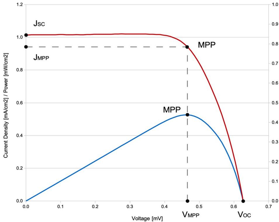
**Figure 2.5:** Typical  $J \times V$  curve of a DSSC.
