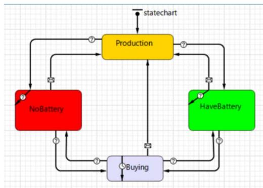
Figure 1: PA state machine during the simulation
