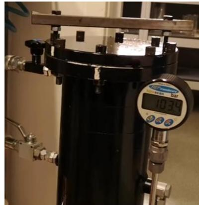
Fig. 2. Pressure testing rig with digital pressure gauge, that is used to perform high pressure tests.
