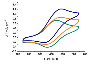
**Figure S-3.** Cyclic voltammograms of (lower curve) gPDH/Os(dmbpy)PVI; (middle curve) dgPDH/Os(dmbpy)PVI and (upper curve) fdgPDH/Os(dmbpy)PVI-modified graphite electrodes in the presence of 10 mM glucose measured in 50 mM PBS pH 7.4 (137 mM NaCl) at a scan rate of 50 mV sec<sup>-1</sup>.
