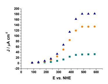
**Figure S-1.** Variation of the catalytic response of ( $\blacksquare$ ) gPDH/Os(dmbpy)PVI; ( $\bullet$ ) dgPDH/Os(dmbpy)PVI and ( $\blacktriangle$ ) fdgPDH/Os(dmbpy)PVI-modified graphite electrodes to 5 mM glucose with the applied potentials measured with the FIA system in 50 mM PBS pH 7.4 (137 mM NaCl) at a flow rate of 0.5 mL min<sup>-1</sup>.
