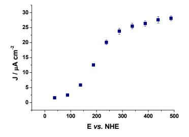
**Figure S-2.** Variation of the catalytic response of fdgPDH/Os(dmobpy)PVI-modified graphite electrodes to 5 mM glucose with the applied potential measured with the FIA system in 50 mM PBS pH 7.4 (137 mM NaCl) at a flow rate of 0.5 mL min<sup>-1</sup>.
