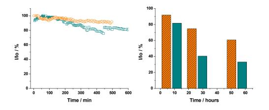
**Figure S-4.** Stability versus time of  $(\circ)$  fdgPDH/Os(dmbpy)PVI and  $(\Box)$  fdgPDH/Os(dmobpy)PVI-modified electrodes measured in the flow-injection mode with 5 mM glucose as substrate. Operational stability is depicted in the left graph; long-term stability is depicted in the right graph. For other conditions see Fig. 4.
