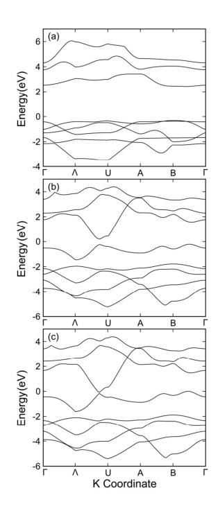
Figure S2. The band structures of NPO tube at various pressures along  $\Gamma(0,0,0) \rightarrow \Lambda(0,1/4,0) \rightarrow U(1/2,1/4,1/2) \rightarrow \Lambda(1/2,0,1/2) \rightarrow B(1/2,0,0) \rightarrow \Gamma(0,0,0)$  in reciprocal space: (a) P = 0 GPa, (b) P = 20 GPa, and (c) P = 25 GPa. The pressure stabilizes the LUMO near the U point as pressure increase because of the P lone pair overlaps between two nearby nanotubes.
