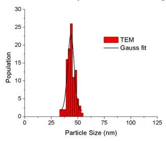
**Figure S1.** Histogram of cit-GNR length using TEM size analysis (taken from 3 images at a resolution of 1.4 pixels/nm). Particle count N = 100; mean = 44.4 nm; std. dev. = 3.9 nm
