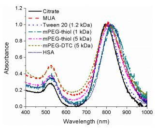
**Figure S3.** Normalized absorbance spectra of surfactant-stabilized GNRs, produced by surface exchange with cit-GNRs using a variety of ligands, surfactants, or proteins. Minor shifts in  $\lambda_{LPR}$  can be observed, consistent with changes in the surface dielectric.
