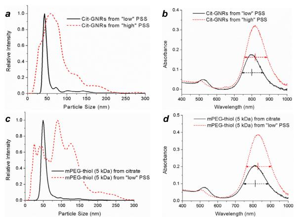
**Figure S2.** NTA plots and vis-NIR spectra of citrate-stabilized GNRs previously suspended in Na-PSS solutions at different concentrations. (a,b) GNRs redispersed in 5 mM Na<sub>3</sub>-cit after 1 C/R cycle from 0.35 wt% Na-PSS ("high") or from < 0.15 wt% Na-PSS ("low"). (c,d) GNRs redispersed in 1.2 mM 5-kDa mPEG-SH after 1 C/R cycle from 5 mM Na<sub>3</sub>-cit or after 1 C/R cycle from "low" PSS.
