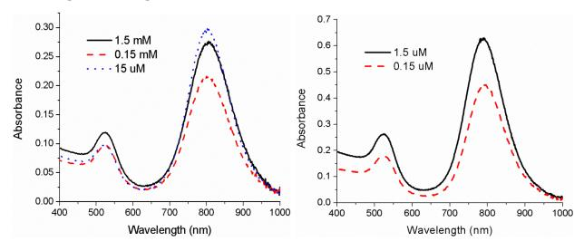
**Figure S4.** Vis–NIR absorbance spectra of cit-GNRs incubated for 12 hours with mPEG-thiol (5 kDa) at loadings ranging from 1.5 mM to 0.15  $\mu$ M. Only minor differences in spectral profile can be discerned, in the visible region ( $\lambda$  < 700 nm).
