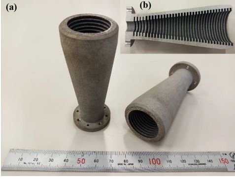
Fig. 1. (a) The as built wideband millimeter-wave corrugated horns fabricated by metal 3D printer (b) The cross section of one corrugated horn cut into two halves.
