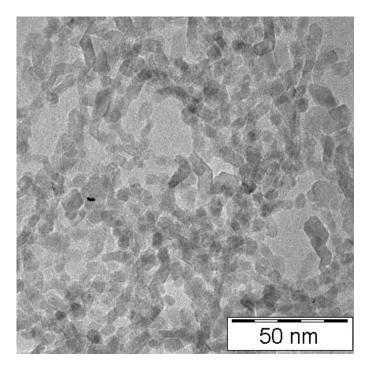
Figure S1. TEM image of SnO<sub>2</sub> nanoparticles.
