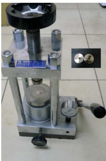
Figure S14 Apparatus ( 769YP-15A powder compressing machine ) for the pressure sensing of S-xerogel of N3 .
