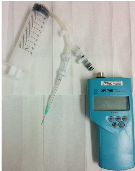
Figure S3. Depiction of leak and burst pressure testing device. Bifurcated tubing from a syringe leads to a digital manometer and a needle. The needle is inserted into clamped intestine and filled with saline solution. Simultaneously, the pressure is recorded when leakage first occurs from the intestine (leak pressure) and at the maximum pressure reached (burst pressure).
