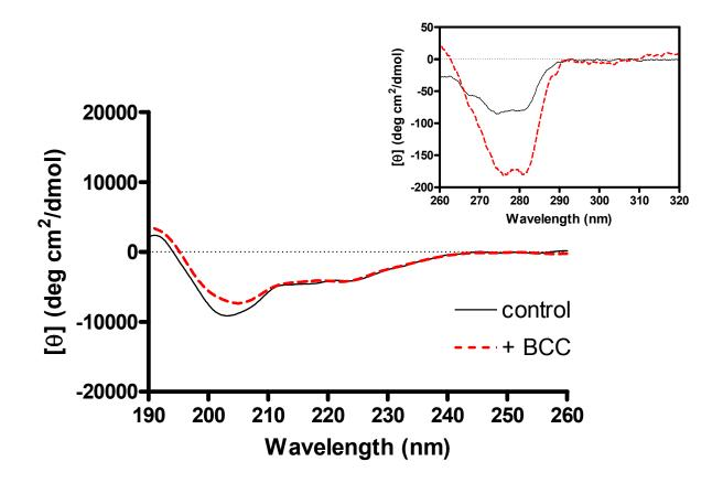
Figure S8. Far-UV CD spectra of CEEP in the presence or absence of BCC at pH 7.4. The concentration of CEEP and BCC were 50  $\mu$ g/ml and 300  $\mu$ g/ml, respectively. The inset shows the near-UV CD spectra of CEEP in the presence or absence of BCC at pH 7.4. The concentration of CEEP and BCC were 300  $\mu$ g/ml and 2 mg/ml, respectively.
