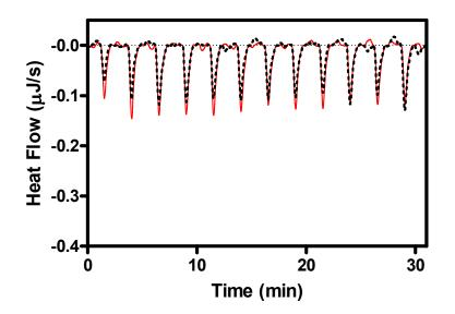
Figure S5. Isothermal titration calorimetry for BCC (6  $\mu$ M) injected into CEEP (100  $\mu$ M) at pH 7.4. Each peak in heat flow chart corresponds to the injection of 2.5  $\mu$ L aliquots of BCC at 25 °C (solid line). The heats of dilution were depicted in control titrations by injecting BCC solution into pure buffer (dotted line).
