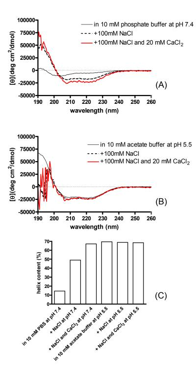
Figure S2. (A) Effects of salt ion on Far-UV CD spectra of CEEP at pH 7.4. (B) Effects of salt ion on Far-UV CD spectra of CEEP at pH 5.5. (C)  $\alpha$ -Helix contents of CEEP calculated from  $[\theta]_{222}$  at various solvent conditions were shown.
