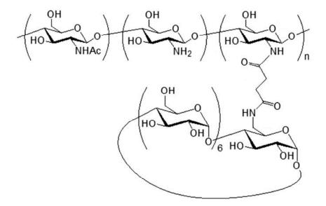
Figure S1. The structure of  $\beta$ -cyclodextrin-grafted chitosan (BCC). The averaged molecular weight was determined from the elemental analysis as 30,800, and  $\beta$ -CyD-content was calculated as 8.0% by NMR, which means  $\beta$ -CyD would be grafted to amino group in chitosan per 10 glucosamine units via a succinic linker.
