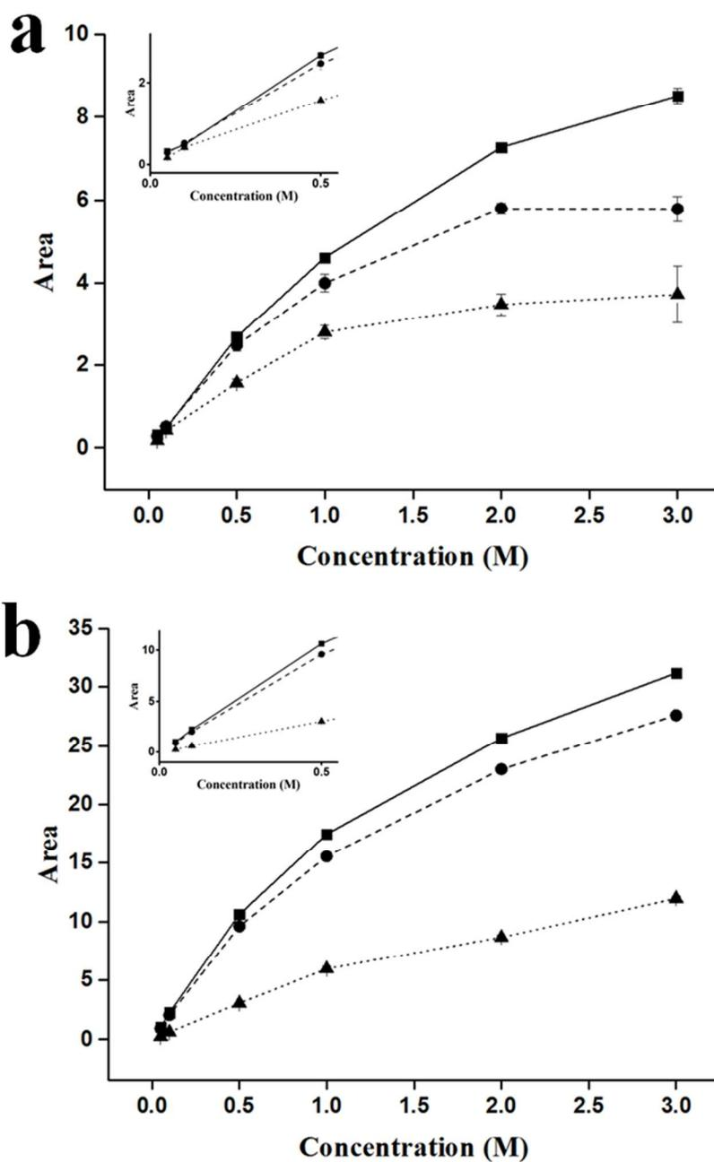
**Figure S4.** Calibration curves of peak areas for concentration of (a) Cl<sup>-</sup> and (b) Na<sup>+</sup> in brine solution from the L<sub>2</sub>-ePt (solid line), Pt black (dashed line), and flat Pt (dotted line) electrodes. The conditions for ion chromatography are the same as those for Figure 9. The error bars are based on the standard deviations from four independent measurements for respective points.
