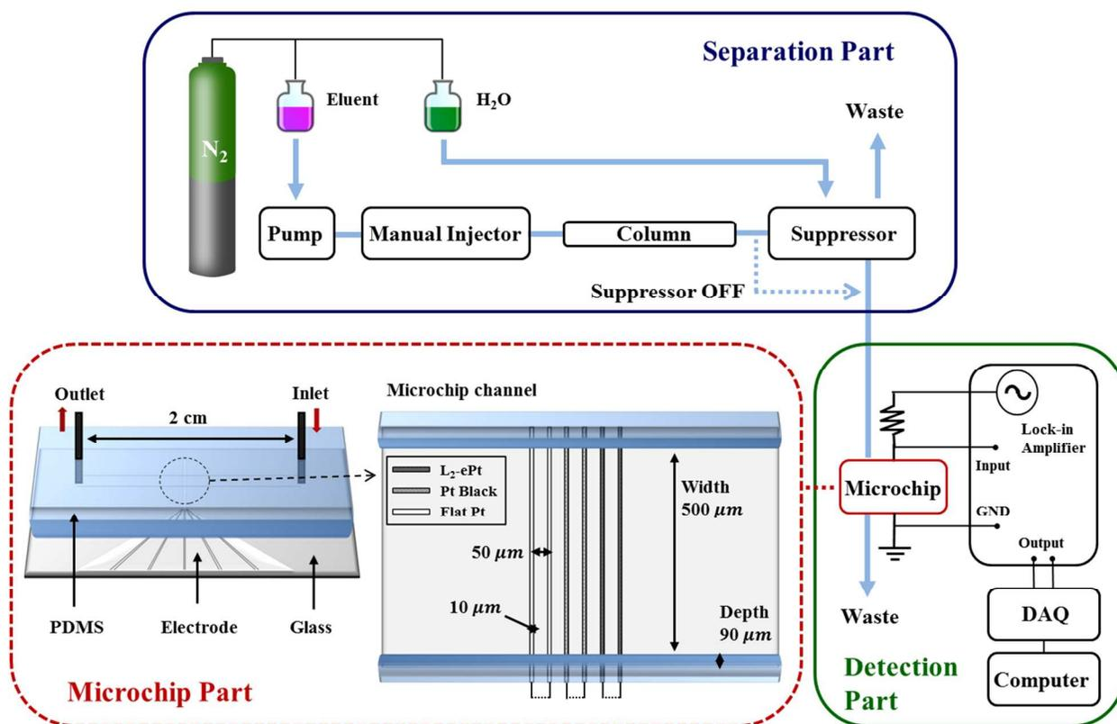
**Figure S2.** Schematic diagram of the setup used for ion chromatography with microchip-based conductivity detector.
