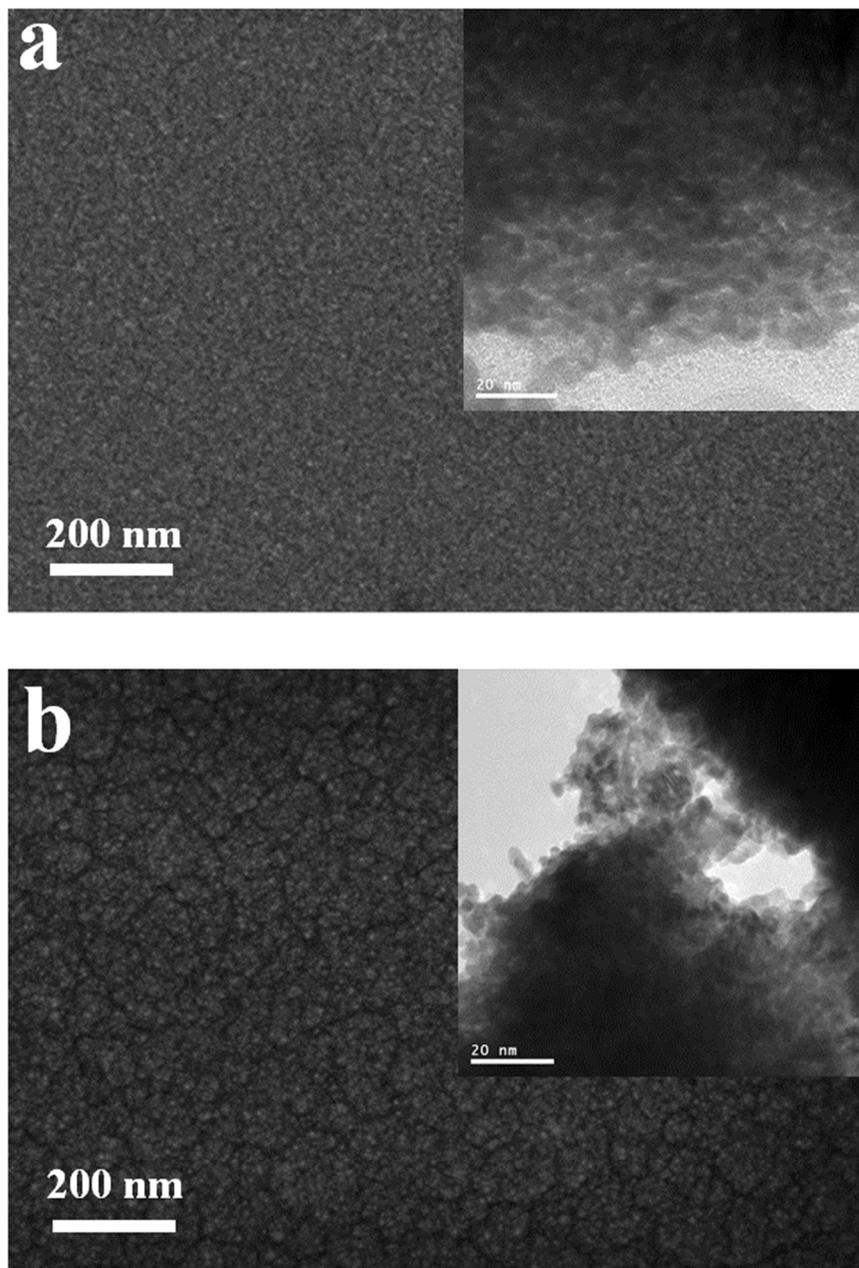
**Figure S1.** SEM and TEM (inset) images of nanoporous Pt electrodes: (a) L<sub>2</sub>-ePt and (b) Pt black.
