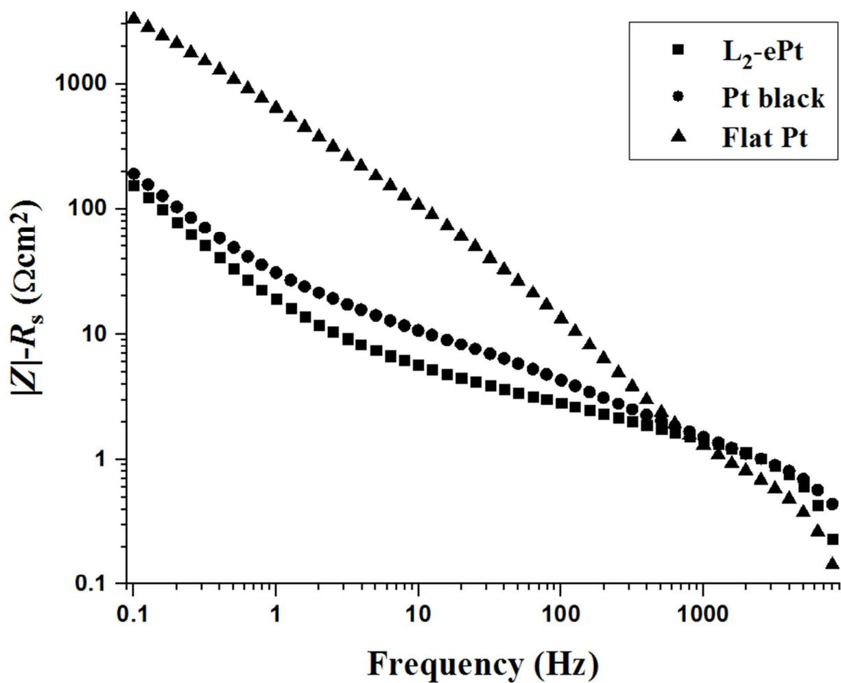
**Figure S3.** Electrode impedance as a function of frequency in 1 mM NaF solution.
