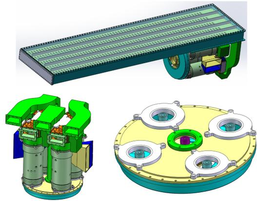
Fig. 11. High-power phase-shifter.
