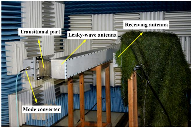
Fig. 14. Measurement of the leaky-wave antenna.
