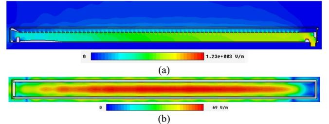
Fig. 6. (a) Electric field distribution inside the slotted waveguide. (b) Electric field distribution on the dielectric plate surface.
