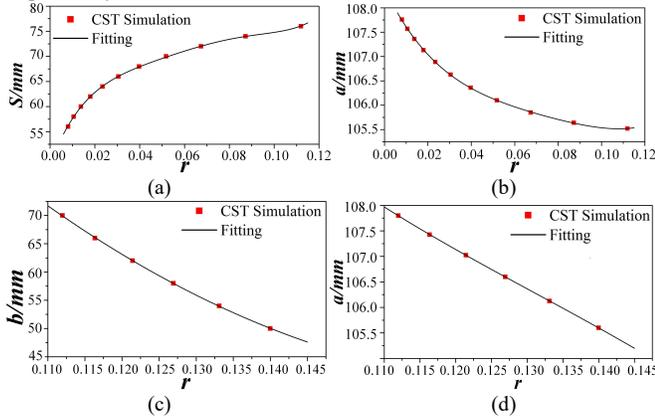
Fig. 3. Structural parameters versus the equivalent resistance. (a,b)  $b=70$  mm. (c,d)  $S=77$  mm.
