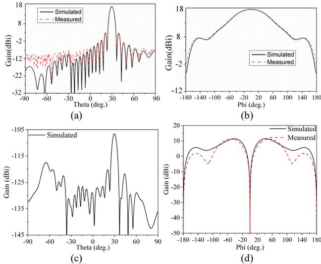
Fig. 16. (a) Co-polar radiation pattern on E-plane. (b) Co-polar radiation pattern on H-plane. (c) Cross-polar radiation pattern on E-plane. (d) Cross-polar radiation pattern on H-plane.
