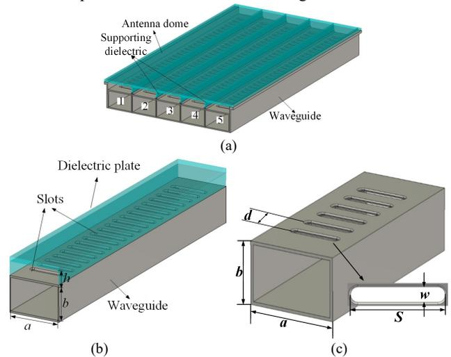
Fig. 1. Configuration of the leaky-wave array antenna. (a) The whole array. (b) Single waveguide. (c) Slots arrangement.
