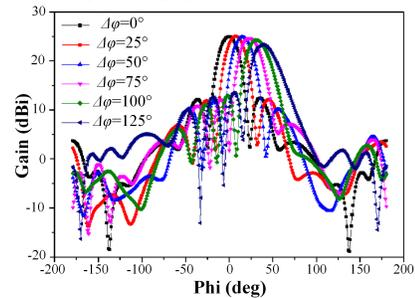
Fig. 12. Simulated radiation pattern of the array antenna.
