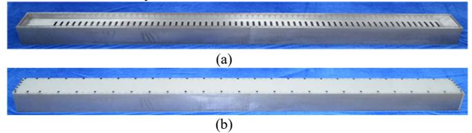
Fig. 13. Photograph of the leaky-wave antenna. (a) Without dielectric cover. (b) With dielectric cover.
