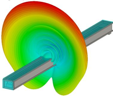
Fig. 9. Simulated 3-D radiation pattern of the single antenna.
