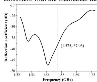
Fig. 7. Reflection coefficient of the antenna.
