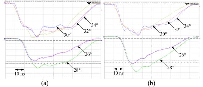
Fig. 18. Detected microwave of the HPM source. (a) Radiation power is 1.3 GW. (b) Radiation power is 1.5 GW.
