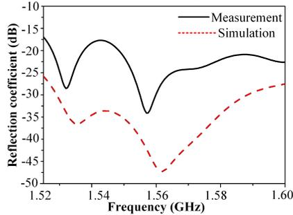
Fig. 15. Measured reflection coefficient of the leaky-wave antenna.
