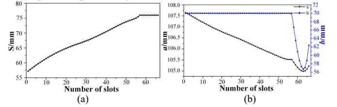
Fig. 5. (a) Length of each slot. (b) Waveguide width and height corresponding to each slot.
