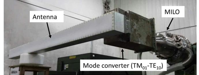
Fig. 17. Device of high-power experiment.
