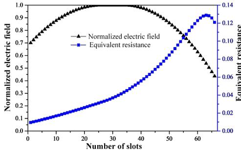
Fig. 4. Aperture distribution of the antenna and the equivalent resistance of each slot.
