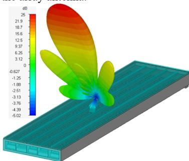
Fig. 10. Simulated 3-D radiation pattern of the array antenna.
