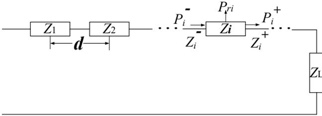
Fig. 2. The equivalent circuit of the leaky-wave antenna.
