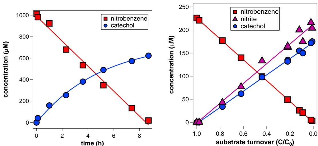
**Figure S3** Left: kinetics of nitrobenzene (red squares) and catechol (blue circles) during transformation in crude cell extract. Right: concentrations of nitrobenzene (red squares), nitrite (purple triangles), and catechol (blue circles) during transformation by purified NBDO.
