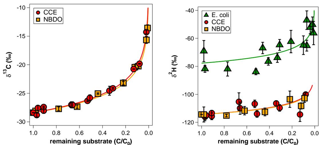
**Figure S4** Left: carbon isotope signatures of nitrobenzene versus remaining substrate concentration for experiments with crude cell extract (red circles) and purified NBDO (yellow squares). Right: hydrogen isotope signatures of nitrobenzene versus remaining substrate concentration for experiments with *E. coli* clones (green triangles), crude cell extract (red circles) and purified NBDO (yellow squares).
