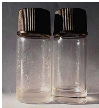
Figure S4. The \text{CH}_2\text{Cl}_2 solution of PAMA resulted from radical polymerization with AIBN as initiator (left) and by lewis pair polymerization with \text{Al}(\text{C}_6\text{F}_5)_3/\text{Dip-IPr}=\text{CH}_2 as catalyst (right).
