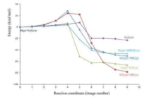
Figure S1. Minimum energy pathways for the reactions of  $H(g) + Si_2H_5(a)$  as the function of proper reaction coordinate.
