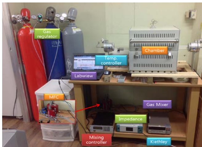
Figure S5. Homemade setup for gas sensitivity measurement
