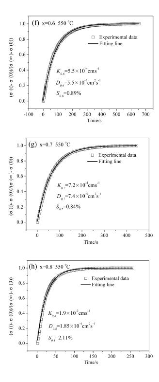
Figure S1. Experimental data and fitting curves of conductivity change profiles as a function of relaxation time for  $La_{0.8-x}Bi_xSr_{0.2}FeO_{3-\delta}$  ( $0 \le x \le 0.8$ ). (a) x = 0 and 0.1 at 800 °C. (b) x=0.2, (c) x =0.3, (d) x =0.4, (e) x =0.5, (f) x =0.6, (g) x =0.7, and (h) x
