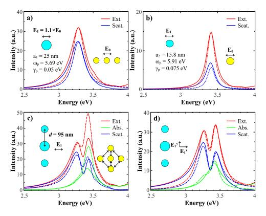
Figure S2: Dipolar fitting for the silver trimer (a) and individual particle (b), and calculated cross sections for the coupling dipolar scatters under transverse (c) and slant (d) excitations. The cross sections are normalized by  $\pi a_0^2$  ( $a_0 = 25$  nm), and the dashed lines are the fitted spectra.
