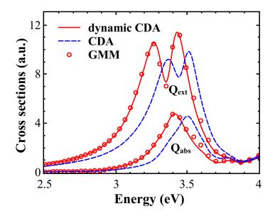
Figure S1: Optical cross sections for the silver pentamer as illustrated in Fig. 2 calculated by CDA and GMM method.
