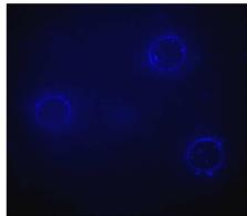
**Figure S1.** Example of microwells created by puncturing a PDMS film (100 μm thickness) with a micropipette for the observation by fluorescence of small populations of isolated mitochondria (autofluorescence of endogenous NADH).
