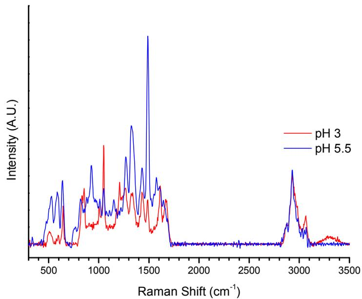
Figure S3. Complete Raman spectra showing normalization to C-H region from 2800-3000 cm<sup>-1</sup>.
