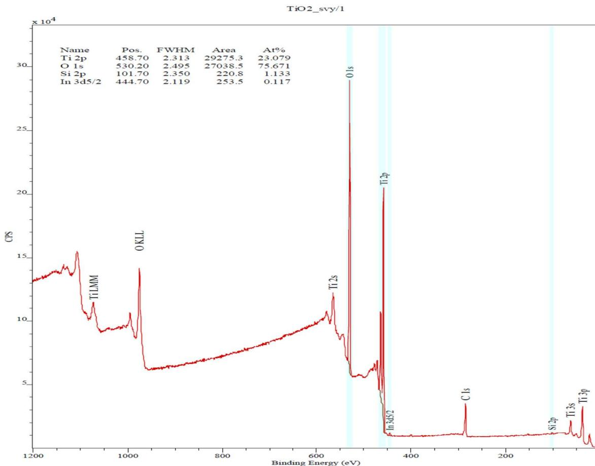
Figure S1. XPS spectra of a TiO<sub>2</sub> layer (10 nm thick) deposited on a mica surface.
