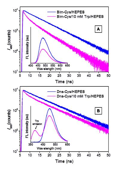
**Figure S5.** Fluorescence decay curves and steady-state spectra of the model compounds (A) Bim-Cys and (B) Dns-Cys both with and without 10 mM L-tryptophan (Trp) in a 25 mM HEPES buffer at pH 7.4.
