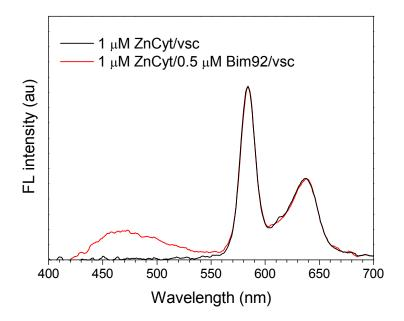
**Figure S9.** Fluorescence spectra ( $\lambda_{ex}$  = 386 nm) of ZnCyt with and without added Bim92 in the presence of TOCL/DOPC liposomes (50 mol % CL, 750 µM total lipid).
