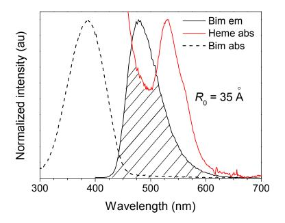
**Figure S1.** Spectral overlap of Bim-Cys emission and cyt *c* ferric heme absorption. The critical distance,  $R_0$ , was calculated to be 35 Å according to Eq. S2.
