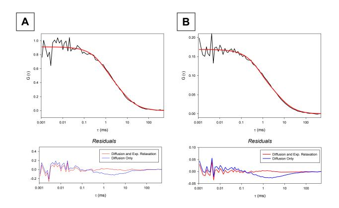
**Figure S10.** Autocorrelation curves of Bim92 cyt *c* in a 25 mM HEPES buffer at pH 7.4 with TOCL/DOPC vesicles (50 mol % CL). (A) 10 nM protein and 750  $\mu$ M total lipid and (B) 50 nM protein and 75  $\mu$ M total lipid. Lower panels show fit residuals of the corresponding autocorrelation curves with (*red*) and without (*blue*) an exponential relaxation term.
