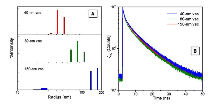
**Figure S8.** (A) Size distribution of TOCL/DOPC (50 mol % CL, 750  $\mu$ M total lipid) liposomes and (B) TR-FRET decay curves of liposome-bound Bim92 with different radii in a 25 mM HEPES buffer at pH 7.4.
