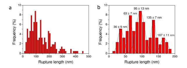
Supplementary Figure 1. Rupture length of the zipper interaction. (a, b) Histograms of the rupture distances of force plateaus measured between an amyloid-tip and an Ig-T surface, using a pulling speed of 200 nm/s and an interaction time of 250 ms (data from Figure 2). (a) and (b) are the same data expressed at different scales. The histogram in (b) shows that many force plateaus ruptured at distances corresponding to multiples of 30 nm, the length of a fully stretched T region.
