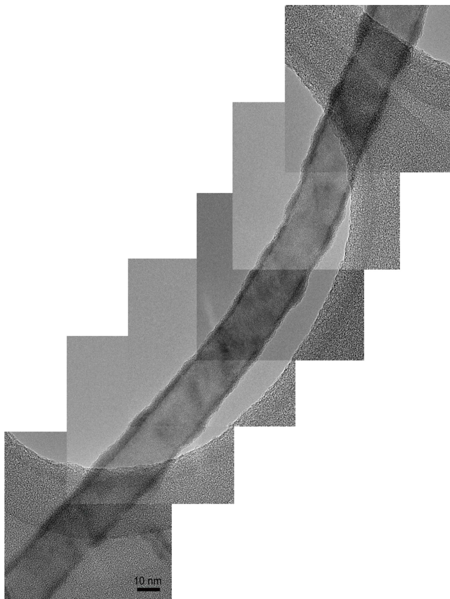
Fig. S2 A series of TEM images of uniform Ge shell deposition along the 320 nm long Si core. The measured shell thickness is 2 \pm 0.6 nm.
