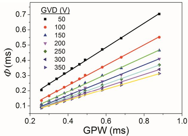
**Figure S-3.** Linear fitting of the GPW contribution to fwhm  $\Phi$  as a function of GPW at different GVD levels.
