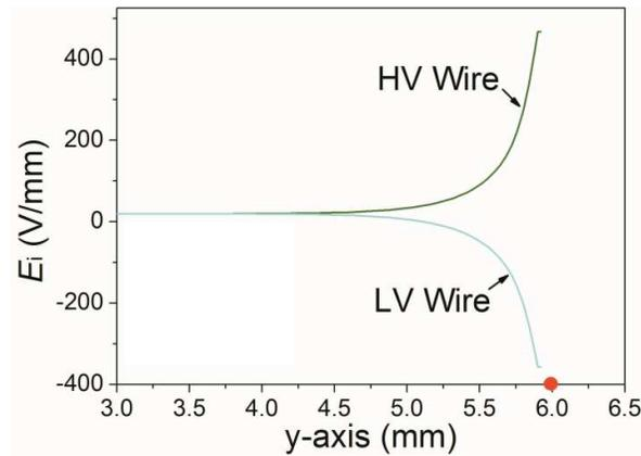
**Figure S-1.** BN gate induced electric field  $E_i$  at different injection electric fields  $E_0$  of 100, 200, 300, 400 and 500 V/cm after the high- and low- voltage gate wires, showing that  $E_i$  doesn't change with  $E_0$ .
