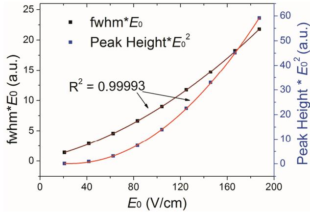
**Figure S-2.** Fitting of the product of the fwhm and  $E_0$ , and the product of peak height by  $E_0^2$ , as a quadric function with  $E_0$  with  $R^2 > 0.9999$ .
