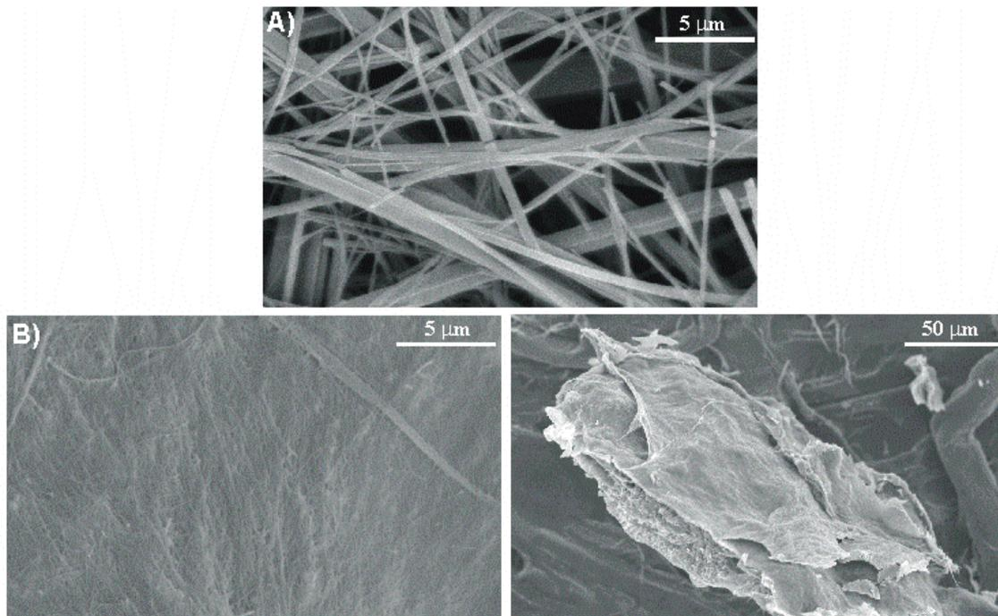
**Figure B.** SEM images at different magnifications of A) DF-OMe after heating at 403 K, B) DF DKP - (DF-OMe after heating at 463 K).
