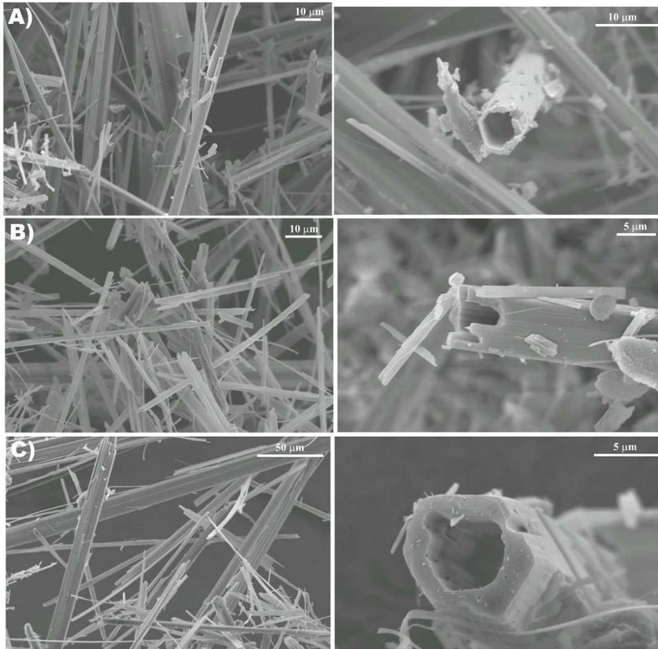
**Figure A.** SEM images at different magnifications of A) FF nanotubes after removing water, B) FF nanotubes after water diffusion and C) FF nanotubes after methanol diffusion.
