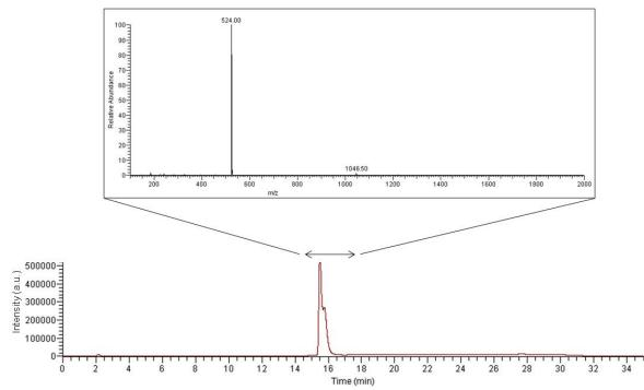
**Figure S5.** LC/MS analysis of ceftiofur after immersion of a drug-loaded organogel in PBS for 48 h. The bottom part of the figure shows the chromatogram of the extracted ceftiofur Na while the inset shows the combined mass spectrometry data of the region spanning 14–17.5 min.
