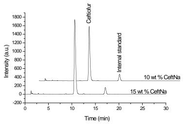
**Figure S4.** Chromatograms of ceftiofur·Na loaded in BTyrOMe gels and stored for 3 months at 4 °C. Gels were loaded with either 10 or 15 wt % drug.
