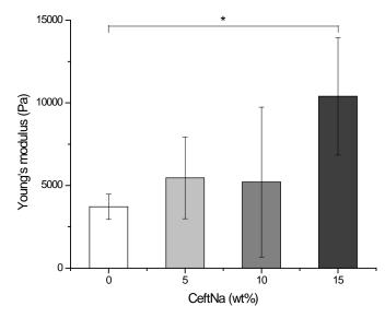
**Figure S11.** Effect of ceftiofur·Na loading on the Young's modulus of organogels. The organogels were composed of 0.1 mmol.g<sup>-1</sup> BTyrOMe, 0.3 mmol.g<sup>-1</sup> NMP, and increasing amounts of ceftiofur·Na in safflower oil. The NMP was allowed to diffuse out of the gels for 24 h at 37 °C prior to mechanical testing. Mean  $\pm$  SD (n = 2-6). \*p < 0.05
