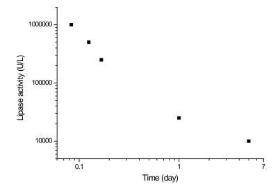
**Figure S3.** Time for complete disintegration of  $400 \,\mu\text{L}$  BTyrOMe organogels. The organogels were incubated at 37 °C in PBS pH 7.4 in presence of increasing concentrations of lipase. The organogels were composed of 0.01 mmol BTyrOMe and 0.03 mmol NMP per gram of safflower oil.
