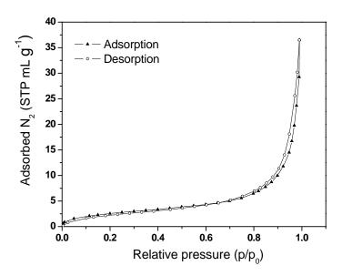
**Figure S1:** Nitrogen adsorption/desorption isotherms of a macroporous foam made of poly(furfuryl alcohol). The large increase of adsorbed  $N_2$  at high pressure is related to macroporosity. However, the small hysteresis cycle and the small adsorption at low pressure indicate very little mesoporosity and microporosity, respectively. Therefore, the material is mainly macroporous.
