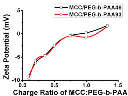
Figure S1. Zeta-potential of spherical aggregates with various charge ratios.
