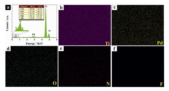
**Figure S2.** (a) EDX spectrum of Pd/TiO<sub>2</sub> NTs; EDX elemental mapping of (b) Ti, (c) Pd, (d) O, (e) N, and (f) F on the top surface.
