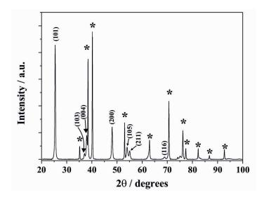
Figure S1. XRD pattern of TiO<sub>2</sub> NTs annealed at 450 °C for 1h.
