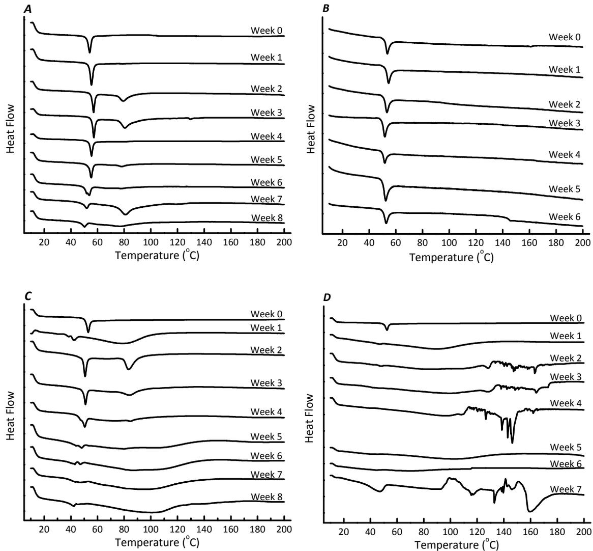
**Figure S6.** DSC thermograms of **poly LG(26k)** (A), **poly LG(16k)** (B), **R-SAP** (C) and **R-ROP** (D) as a function of degradation time. Note: weeks 5,6,7 for (D) are omitted in the figure in the main article because the sample size was sufficiently small after 4 weeks of degradation to make the data traces unreliable. The thermograms for **poly LG(26k)** and **R-ROP** (weeks 1-4) are repeated here to facilitate comparison.
