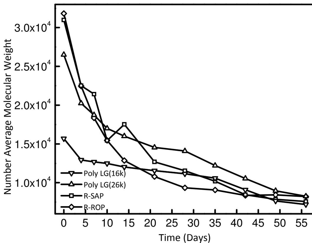
**Figure S4.** The number average molecular weight ( $M_n$ ) decrease as a function of degradation time. The figure in the main body of the paper has been normalized relative to initial molecular weight.
