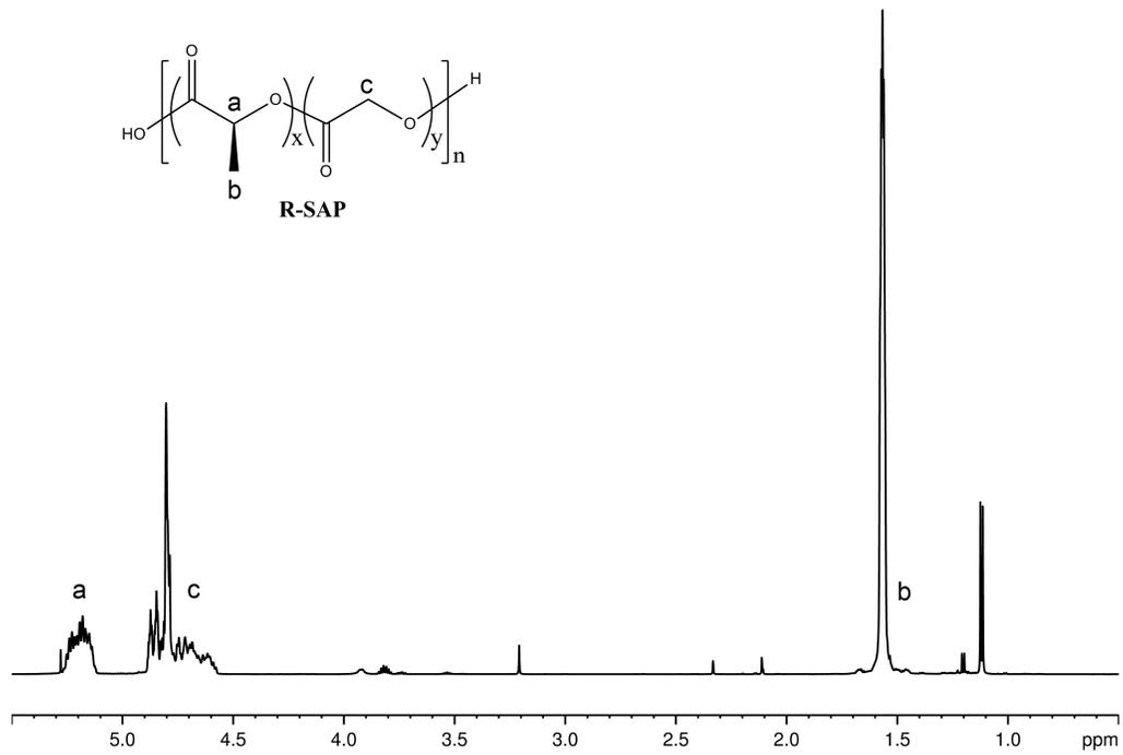
**Figure S1.**  $^1\text{H}$  NMR (600 MHz,  $\text{CDCl}_3$ ) spectrum of R-SAP.
