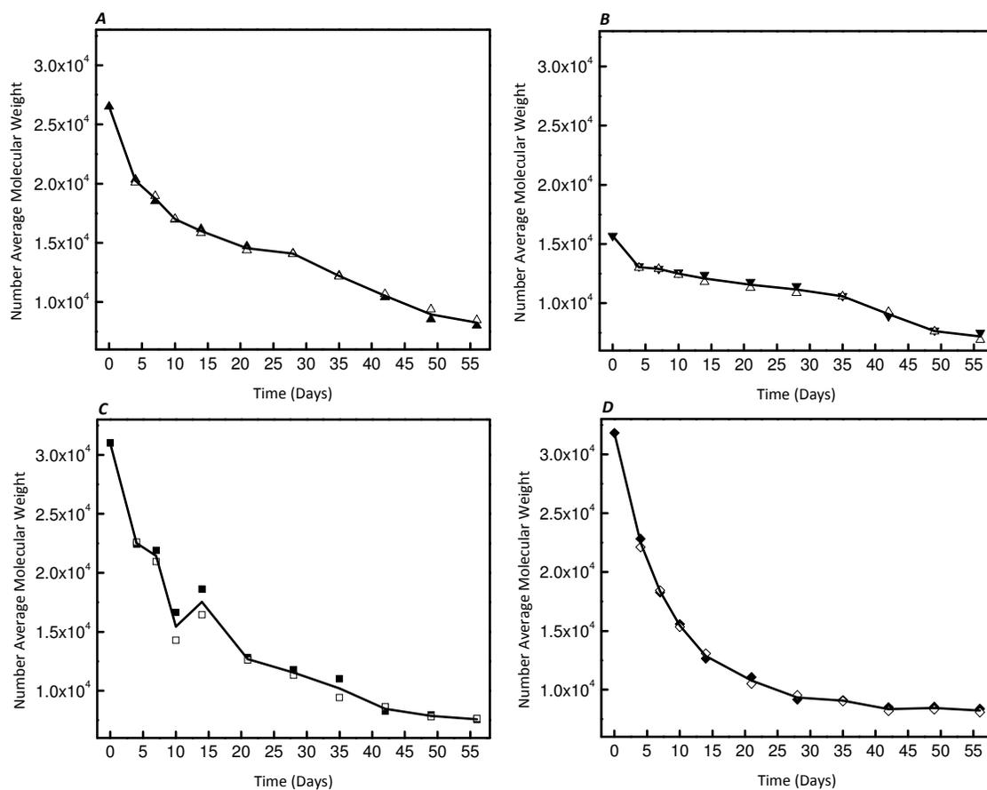
**Figure S5.** The spread of number average molecular weight ( $M_n$ ) decrease of **poly LG(26k)** (A), **poly LG(16k)** (B), **R-SAP** (C) and **R-ROP** (D) as a function of degradation time. The solid symbols and open symbols represent independent experiment results. The line is plotted by the average of  $M_n$  from each experiment result.
