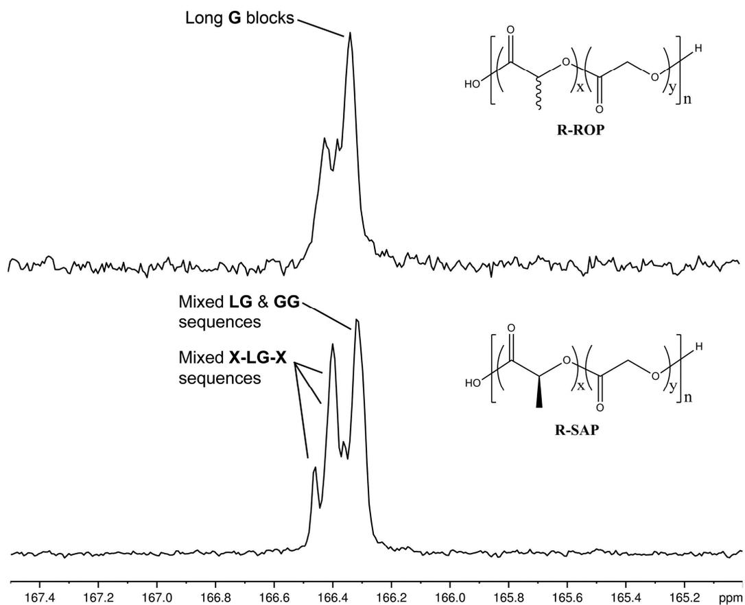
**Figure S3.** Comparison of glycolyl carbonyl resonances for **R-ROP** (top) and **R-SAP** (bottom). The X represents either L or G units.
