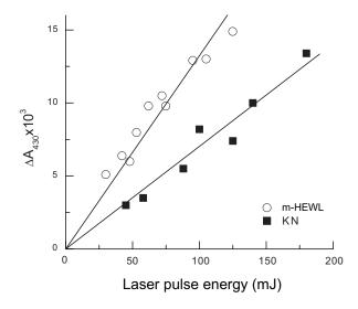
The laser pulse energy dependencies of the initial absorption values measured at 430 nm in flash photolysis of m-HEWL and KN neutral aqueous solutions. Both sample had the same absorption at 355 nm.
