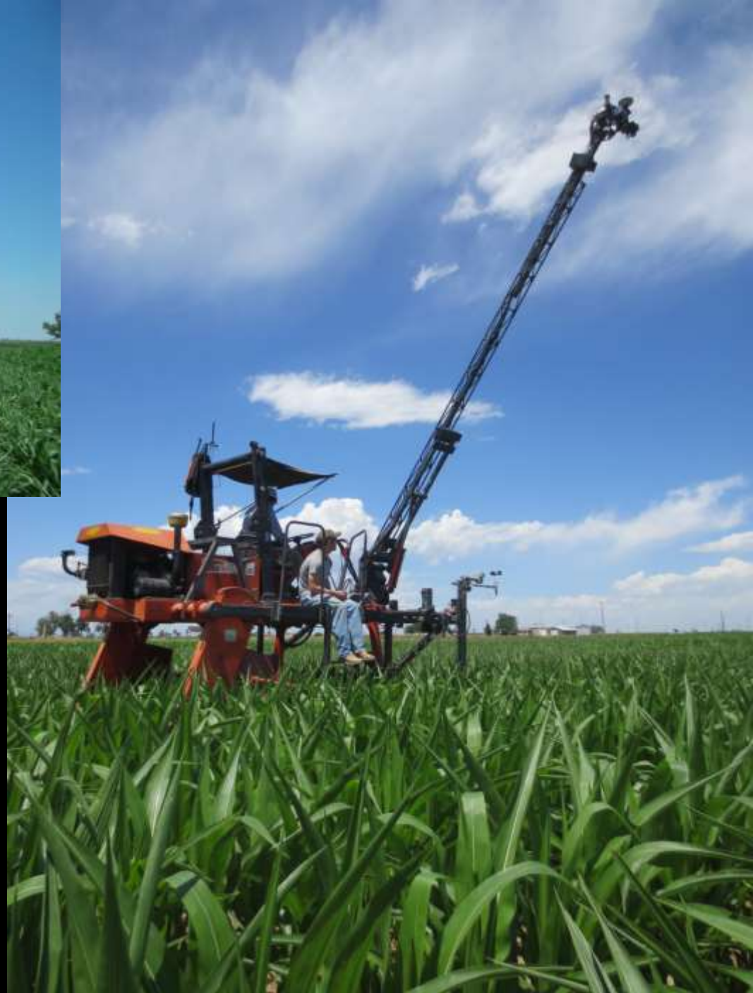
Photo 17. High clearance reflectance tractor taking canopy ground cover images
