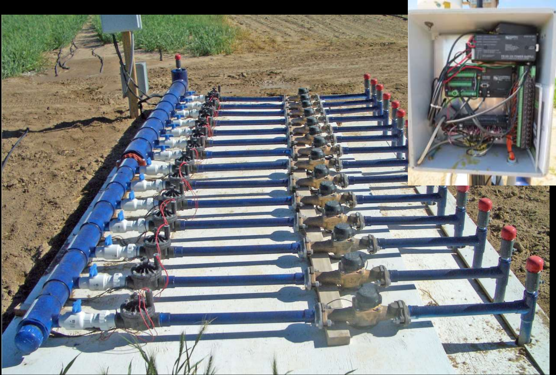
Photo 6. LIRF WPF Trial irrigation control and monitoring system showing hydraulic valves and turbine flow meters for each treatment.
