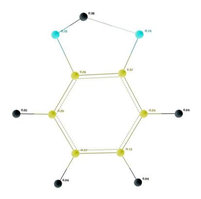
Fig. S-7 – Charge distribution in the hydride adduct at minimum energy.
