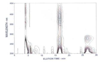
Fig. S-1 – Contour plot of a chromatographic recording fo a solution initially containing 200  $\mu$ M catechol to which 1 equivalent of hexachloroiridate(IV) had been added. The signals at 4.6, 16.5 and 26.8 min represent, respectively, 200  $\mu$ M hexachloroiridate(III), 100  $\mu$ M orthoquinone and 100  $\mu$ M catechol.
