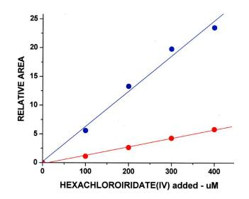
Fig. S-3 - The dependence of mass 109 cation (blue) and anion (red) signals on the concentration of hexachloroirridate(IV) added to 200  $\mu$ M catechol.
