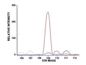
Fig. S-5 – Mass spectra recorded with the MicroMass instrument at the orthoquinone (red) and catechol (blue) peaks. The subtracted background contribution is given by the dotted spectra.
