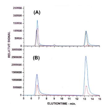
Fig. S-2 – Mass 109 chromatograms for solutions 100 uM in orthoquinone and catechol using (A) electrospray and (B) chemical ionization. <u>Cation</u> signals are in red and <u>anion</u> signals in blue. The dotted red chromatogram in A has been scaled by a factor of 10. Complementary 276 spectrophotometric data, given by the black chromatogram in A identify the mass peaks at 6.7 and 13.2 min as representing orthoquinone and catechol.
