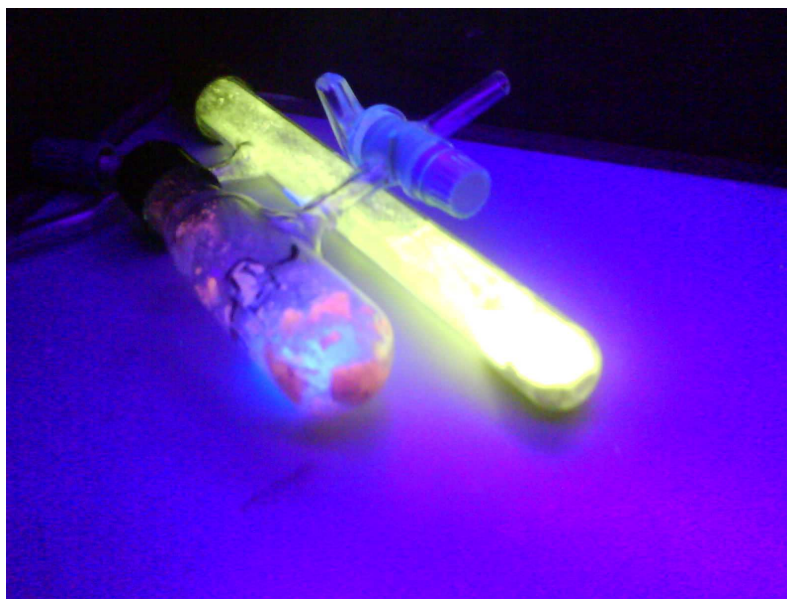
Figure S5. Intense luminescence of [(\text{Et}_2\text{S})_3\{\text{Cu}_4(\mu_3\text{-I})_4\}]_n (right Schlenk tube) and [(\text{THT})_2\text{Cu}(\mu_2\text{-I})_2\text{Cu}(\text{THT})_2] (left Schlenk tube) under UV-light at 366 nm.
