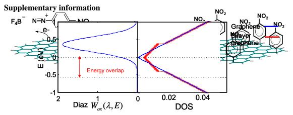
**Figure S1:** Energy overlap of the electronic states of single and bilayer graphene (DOS) and vacant oxidation states of the electron withdrawing species ( $W_{ox}$ ). (Energy overlap is calculated in between the dotted lines.)
