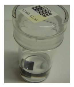
**Figure S4:** Picture of the reactor setup employed for the on chip chemistry. The silicon wafer and the stir bars are at of the bottom of the reactor dipped in water with 17-25 mM 4-nitrobenzene diazonium water and 1 wt% SDS.
