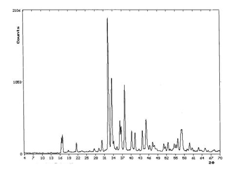
Figure S1. XRD pattern of the obtained powder for monohydrate sodium carbonate.
