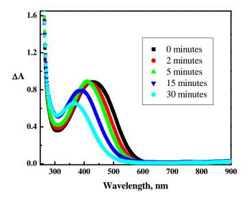
Absorption spectra recorded following the gamma radiolysis of aqueous solution of PTEBS containing 0.1 M NaN<sub>3</sub>. The experimental conditions reflect the reaction of the polymer with azide radicals (reaction 6 in the main text)
