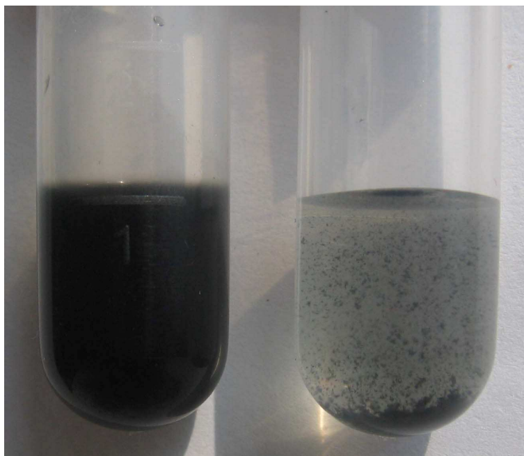
Figure S3 Photograph of PVP-protected graphene (left) and pure graphene (right) dispersed in water.
