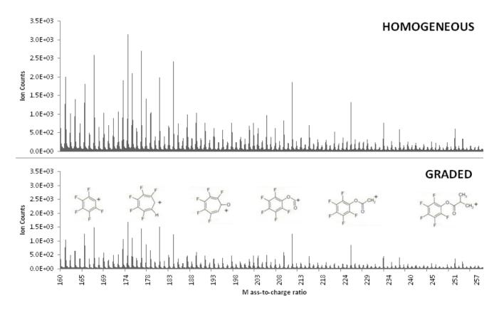
ToF-SIMS spectra of the homogeneous and graded copolymers. Characteristic peaks of the PFM comonomer are highlighted by the accompanying ionic structures.
