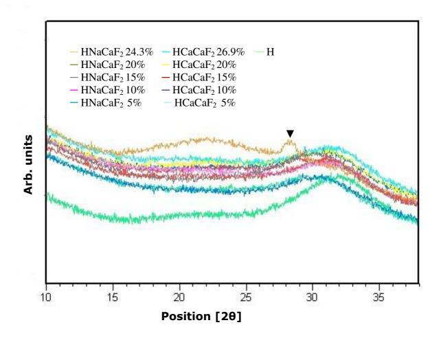
**Figure S1**: The XRD spectra of the as-quenched samples. ( $\nabla = \text{CaF}_2$ )
