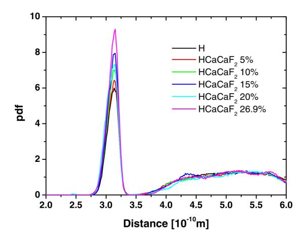
Figure S2:Si-Si Pair Distribution Functions for the HCaCaF<sub>2</sub> glass series.
